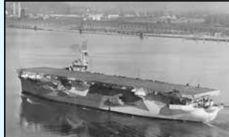
Aircraft carrier escort ship converted from liberty ship, on "trial run" before accepted by Navy for commissioning.
